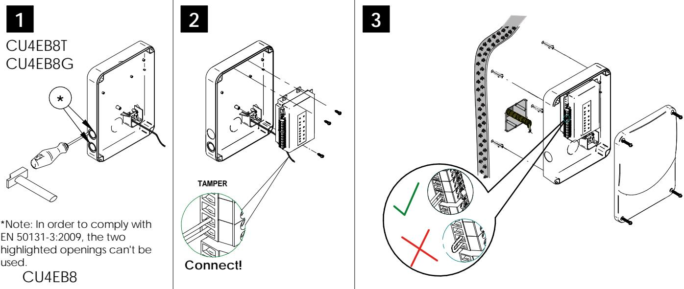
\*Note: In order to comply with EN 50131-3:2009, the two highlighted openings can't be used.
